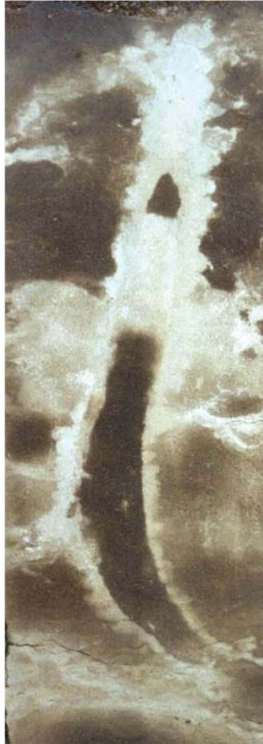
Figure 5.11 Ophiomorpha saturated in oil. No hydrocarbons occur in the impermeable pelletoidal wall. Lower Miocene, Oficina Formation, Oritupano Field, Eastern Venezuela Basin. Core width is 7 cm.
