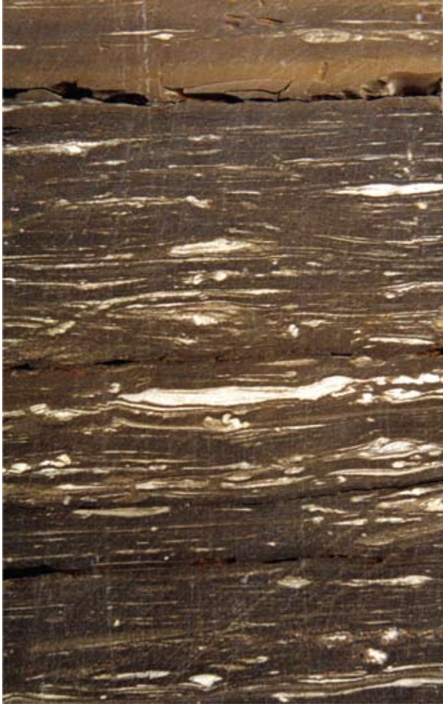
Figure 8.3 Typical core expression of ichnofaunas from central-basin deposits. Note small Planolites , synaeresis cracks, siderite layer (top), and sandstone lenses with very thin mud drapes. Lower Miocene, Oficina Formation, Oritupano Field, eastern Venezuela Basin. Core width is 10 cm.
