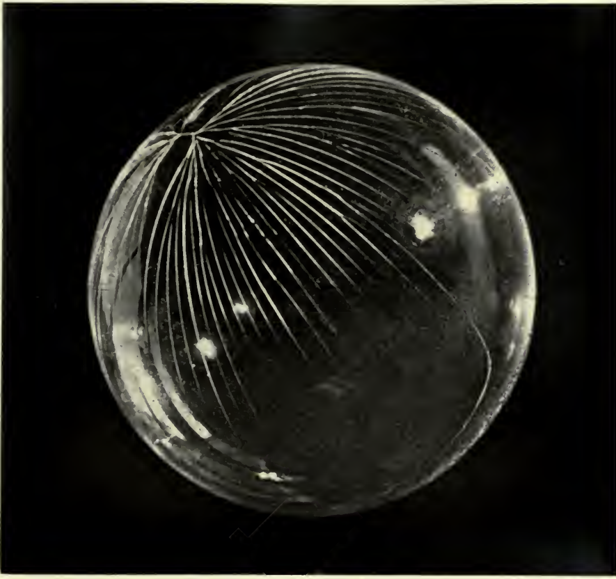
GLASS GLOBE. CRACKED BY INTERNAL PRESSURE ILLUSTRATING THE CAUSE OF THE BRIGHT STREAKS RADIATING FROM TYCHO & s
